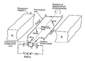
The electric motor is a device which converts electrical energy to mechanical energy. When a rectangular coil is placed in a magnetic field and current is passed through it, forces acts on the coil which rotates it continuously. When the coil rotates, the shaft attached to it also rotates. In this way the electrical energy supplied to the motor is converted into the mechanical energy of rotation.
