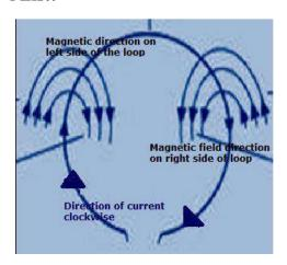
Fleming right-hand rule states that the direction of the magnetic field is perpendicular to the direction of current to flow.
