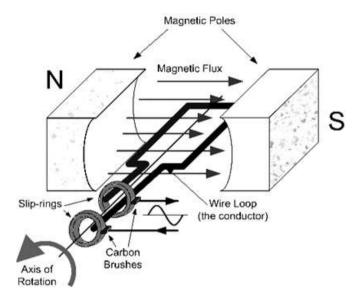
An electric generator is a device that converts mechanical energy obtained from an external source into electrical energy as the output. The flow of electric charges is induced by moving an electrical conductor, such as a wire that contains electric charges, in a magnetic field. This movement creates a voltage difference between the two ends of the wire or electrical conductor, which in turn causes the electric charges to flow, thus generating electric current.
