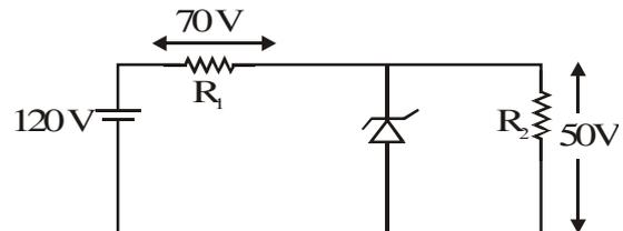
$$\text{Current in } R_1 = \frac{70}{5000} = 14 \text{ mA}$$
