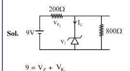
$V_{Z} = 5.6 V$  $V_{R_1} = 9 - 5.6$  $V_{R_1} = 3.4$  $I_{R_1} = \frac{V_{R_1}}{R} = \frac{3.4}{200}$  $I_{R_1} = 17 \text{ mA}$ 200Ω - $R_1$  $I_7$ R<sub>2</sub> **≸**800Ω
