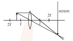
If the whole set up is immersed in water without disturbing the object and the screen position, what will one observe on the screen?
