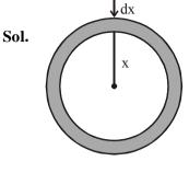
Consider a strip of radius x & thickness dx, Torque due to friction on this strip.
