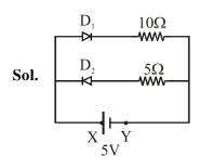
Here only D<sub>1</sub> will work and we know for silicon diode, potential drop on D<sub>1</sub> will be 0.7V
