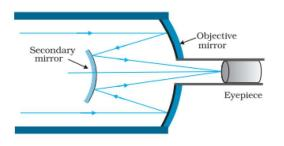
It has advantage of a large focal length in a short telescope
