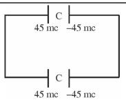
Heat dissipated  $= U_i - U_f$  [Change in energy stored in the capacitors]
