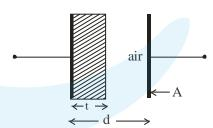
This can be seen as two capacitors in series combination so
